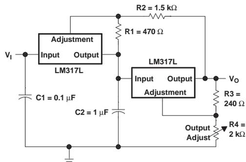
Figure 5. Tracking Preregulator Circuit
