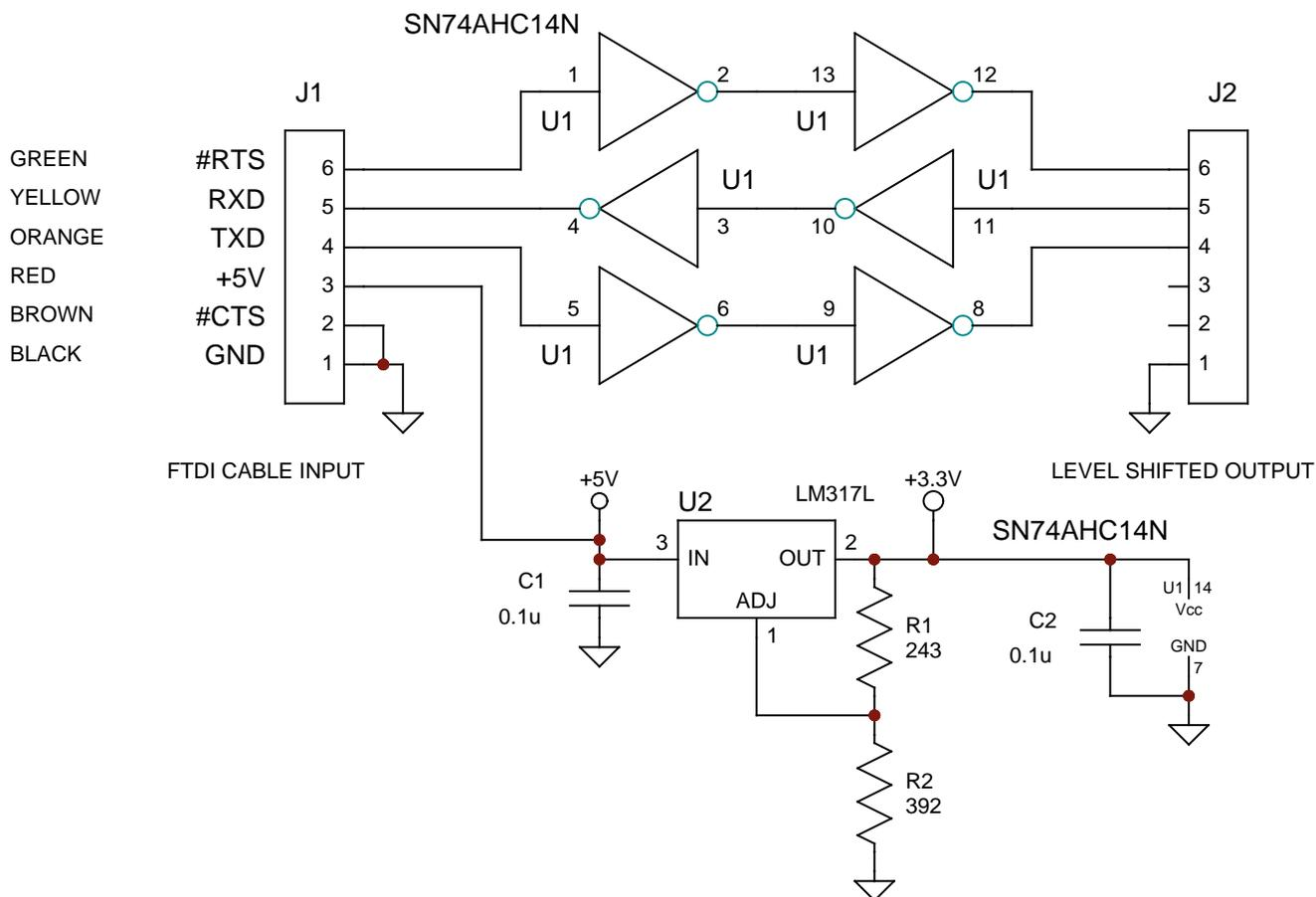
Figure 1: Level Translator for FTDI TTL-232R-5V Cable
